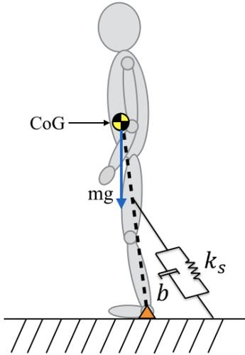
Fig. 1. Graphical representation of the second order muscle-tendon system
