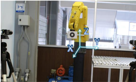
Fig. 2. Calibration of the visual system
