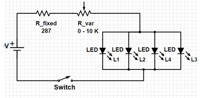
Fig. 2. Current TIS illumination circuit.
