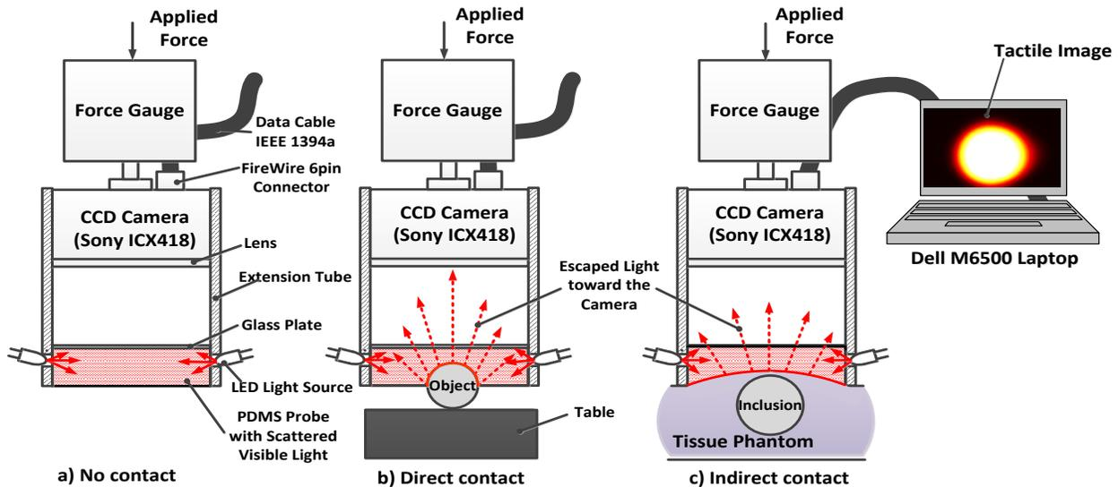
Fig. 1. Tactile Imaging System.
