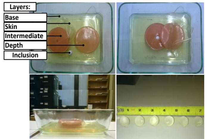
Fig. 6. Tissue phantom and spherical inclusions.
