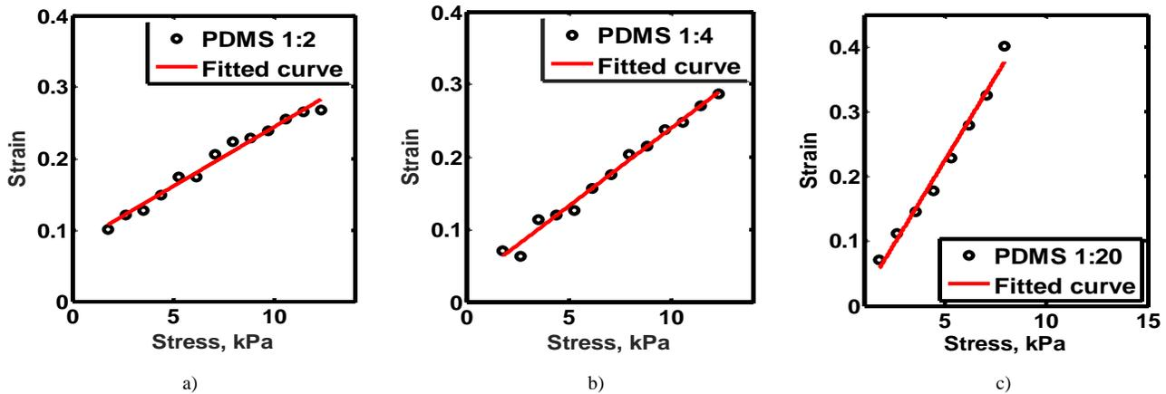
Fig. 7. Stress-strain relationships for the phantom experiments. (a) soft inclusion, (b) medium stiffness inclusion, and (c) stiff inclusion.
