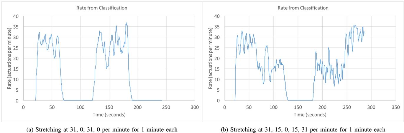
Fig. 3: Rate estimation over time for two experimental runs, computed as the number of actuation classifications made in the past  $k = 6$  seconds extrapolated to a one-minute rate. Note that the plots begin after 20 seconds because the first 20 seconds of data are reserved for training the classifier used in computing the rates.
