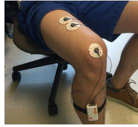
Fig. 3. Placement of EMG Sensor Electrodes
