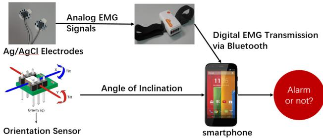
Fig. 4. Architectural Flow Diagram of STS Detection System
