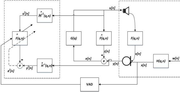
Figure 2. Block Diagram of Proposed AFC Method
