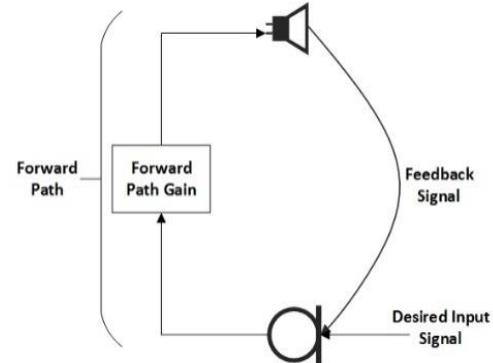
Figure 1. Acoustic coupling between Loudspeaker and Microphone
