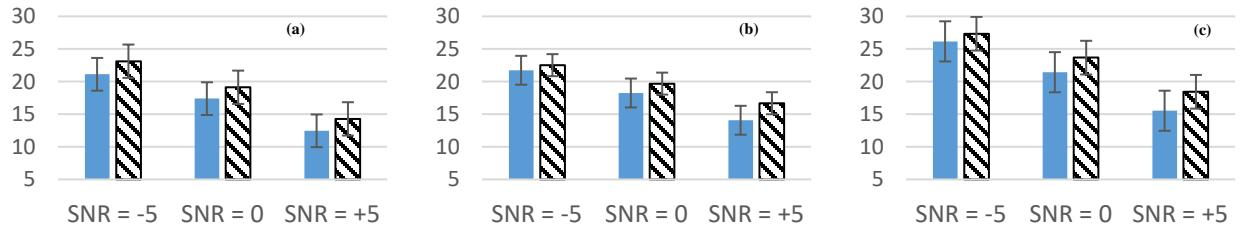
Figure 4. (Left to Right) Signal to Feedback Ratio (SFR) (in dB) plot for PEM-AFC (solid) and Proposed Method (dashed) for (a) Babble, (b) Machinery, and (c) Traffic noise at different SNR (dB) values. Higher SFR is better.
