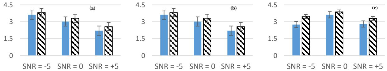
Figure 5. (Left to Right) Perceptual Evaluation of Speech Quality (PESQ) plot for PEM-AFC (solid) and Proposed Method (dashed) for (a) Babble, (b) Machinery, and (c) Traffic noise at different SNR (dB) values. Higher PESQ is better.
