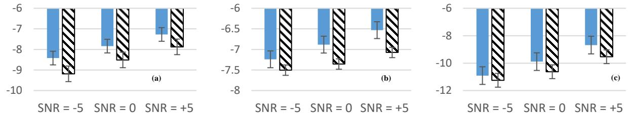
Figure 3. (Left to Right) Misalignment (MISA) (in dB) plot for PEM-AFC (solid) and Proposed Method (dashed) for (a) Babble (b) Machinery, and (c) Traffic noise at different SNR (dB) values. Lower MISA is better
