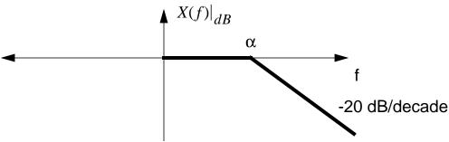
(c) Describe the transfer function for the system that has the following Bode plot (ignore  $\angle X(f)$ ):
