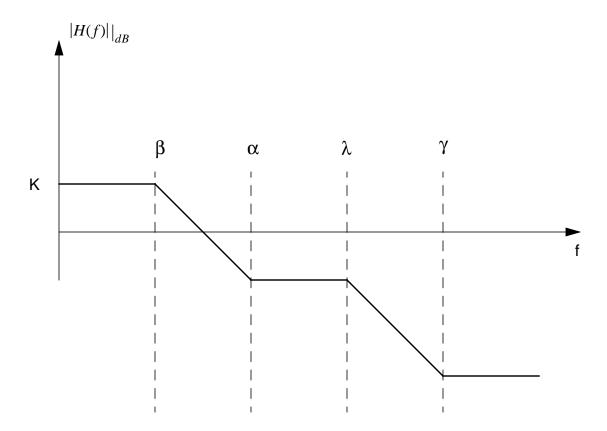
Note that  $K = 20 \log \left( \frac{C\alpha\lambda}{\beta\gamma} \right)$ , and that the slopes of the lines are 20 dB/decade.
