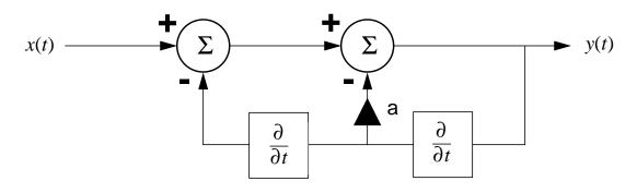
**Problem No. 4**: Use the Routh criterion to determine how many right-half-plane poles the following system has:
