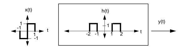
(a) Compute the output, y(t), for the system shown above:
