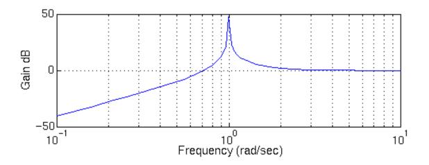
MATLAB code used to generate Bode Magnitude plot: num[1 0 0] den[1 0 1] bode(num,den)
