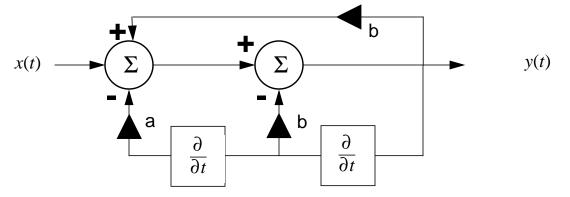
**Problem No. 5**: For the discrete-time system shown, compute the output if the input is given by the sequence  $\{0,1,-1,0,-1,1,0,0,0,...\}$ :
