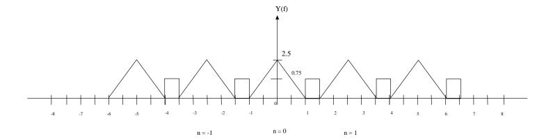
(b) How do you explain the fact that the sample frequency of y(n) is less than the Nyquist rate, yet there is no distortion?
