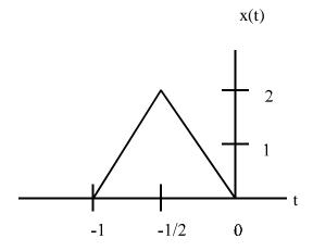
The first portion of the signal is a ramp function. The unit ramp function rises 1 unit per 1 unit run (i.e. slope = rise/run = 1). Since the first portion rises 2 units per  $\frac{1}{2}$  unit run...
