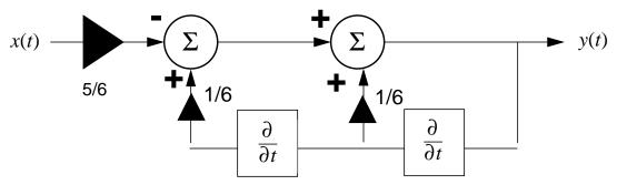
(a) Find the transfer function of this system using Laplace transforms.
