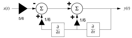
(a) Find the transfer function of this system using Laplace transforms.
