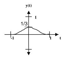
The maximum amplitude is equal to the maximum area shared between x(t) and a convolved h(t). The output is computed by convolution.
