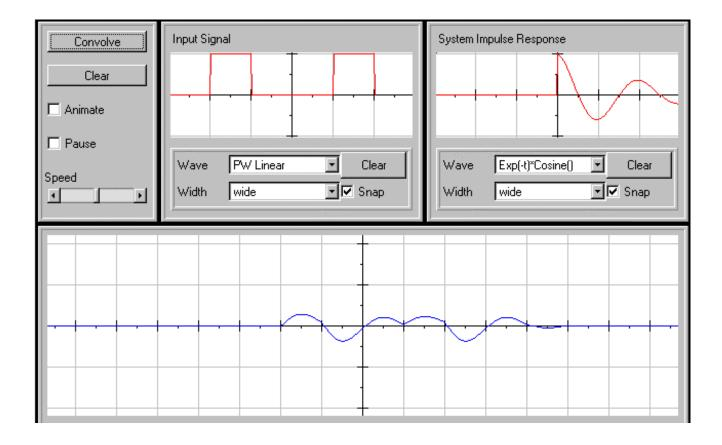
This graph would like the one in part b, but now the output would become periodic. An output identical to part b would occur every 10 seconds.
