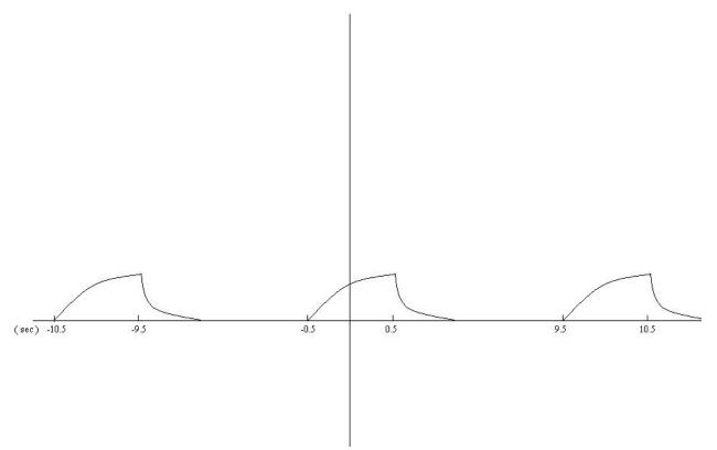
With the period at 10 seconds there is no overlap of the signals. Thus we just have a train of the signal from part b.
