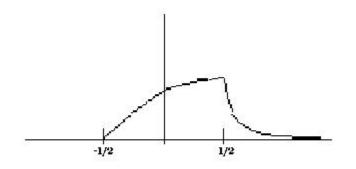
This is the graph of the ouput with the x-axis in seconds. The graph makes sense because with the given circuit, a pulse will cause the circuit to begin to charge like it did with the unit step input. However, when the pulse cuts off after 1 second, the capacitor and inductor will both begin to discharge through the resistor to create the fall-off effect seen above.
