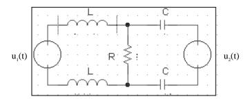
(a) Assume the voltage across the resistor in the circuit above is the output voltage, y(t). Derive the state variables representation of this circuit.
