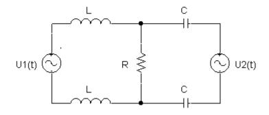
(a) Assume the voltage across the resistor in the circuit above is the output voltage, y(t). Derive the state variables representation of this circuit.
