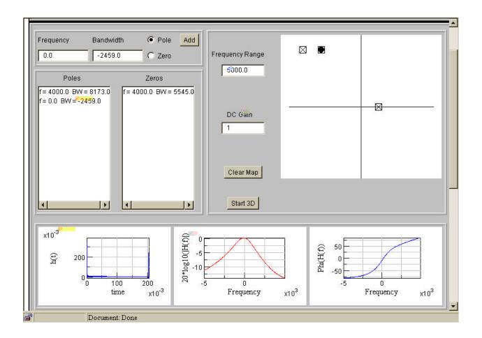
The pole has more of an effect on the frequency response in the s-plane, causing a sharper drop at  $\rm f_S/2.$
