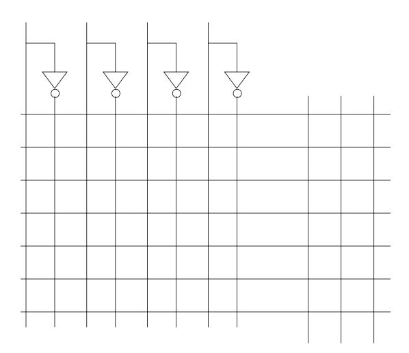
**b)** Suppose that this network was implemented on a ROM. What is the required size of a ROM? What value is stored at the ROM address 1010? What is stored at 0011?
