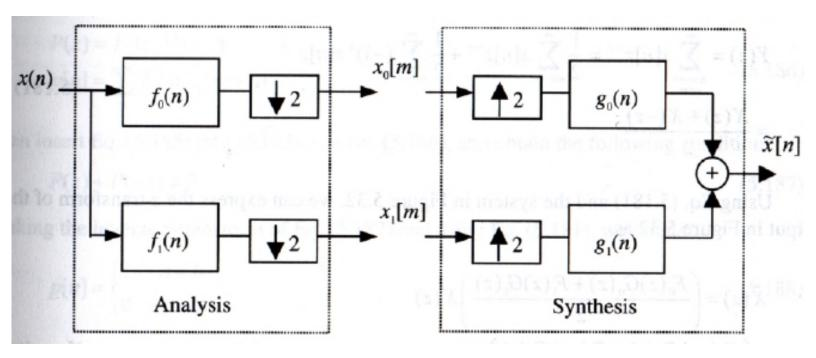
where f(n) and g(n) are complementary low pass and high pass filters:
