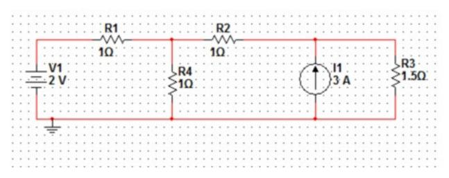
Now simply by using a Parameter Sweep in Multisim we can prove that when RL=Rth we get the maximum power dissipated.
