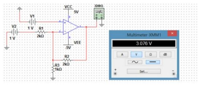
Simply plug in your input voltages in the equation that we derived used KCL. It gives us:  $V_0 = 4(1) - (1)$
