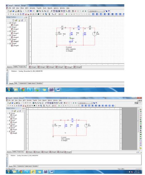
Short the inductors and open the capacitors to begin steady state analysis and redraw the circuit.
