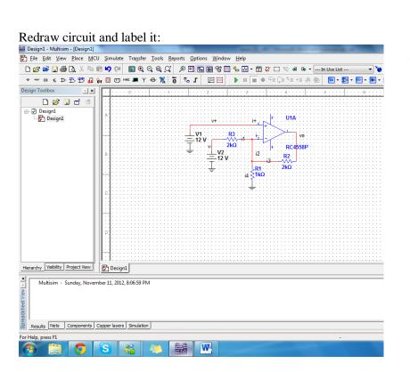
We first write the conditions then apply a KCL and substitute.
