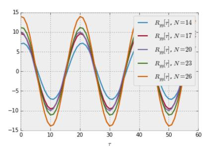
As displayed also in computer assignment 9, the autocorrelation of a signal containing white noise filters out a portion of the noise.
