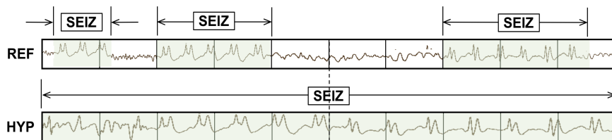
Figure 4. ATWV scores this segment as 0 TP and 3 FN events.
