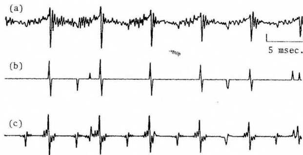
Figure 6. A Comparison Between the MPLPC and the ZMPLPC Excitations: (a) Original Residual (40 msec. Duration); (b) MPLPC Excitation; (c) ZMPLPC Excitation.
