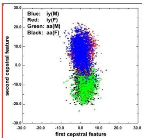
Figure 3. Features used in speech recognition systems exhibit significant overlap in the feature space. Disambiguating these classes requires the use of additional acoustic context.
