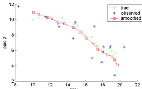
Figure 14. State predictions of an LDM using a traditional Kalman filter.
