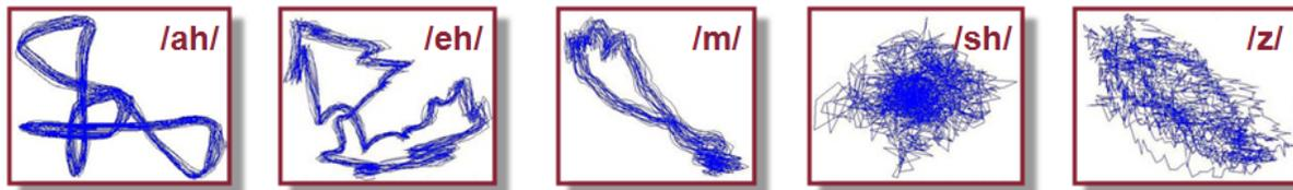
Figure 6. The phase space trajectories of several phonemes. Our goal was to compute a measure of the complexity of the phase space and to use this measure to improve discrimination. For example, a measure of trajectory smoothness should be relatively invariant to changes in acoustic channel or speaker.
