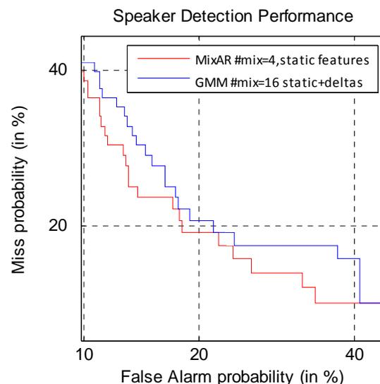
Figure 11. Speaker detection performance (DET curves) for the experiments on the NIST data.
