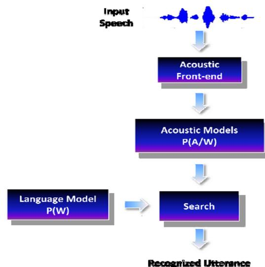
Figure 1. An overview of a typical pattern recognition approach to speech recognition. In this project, we have focused on the acoustic front-end and acoustic modeling.
