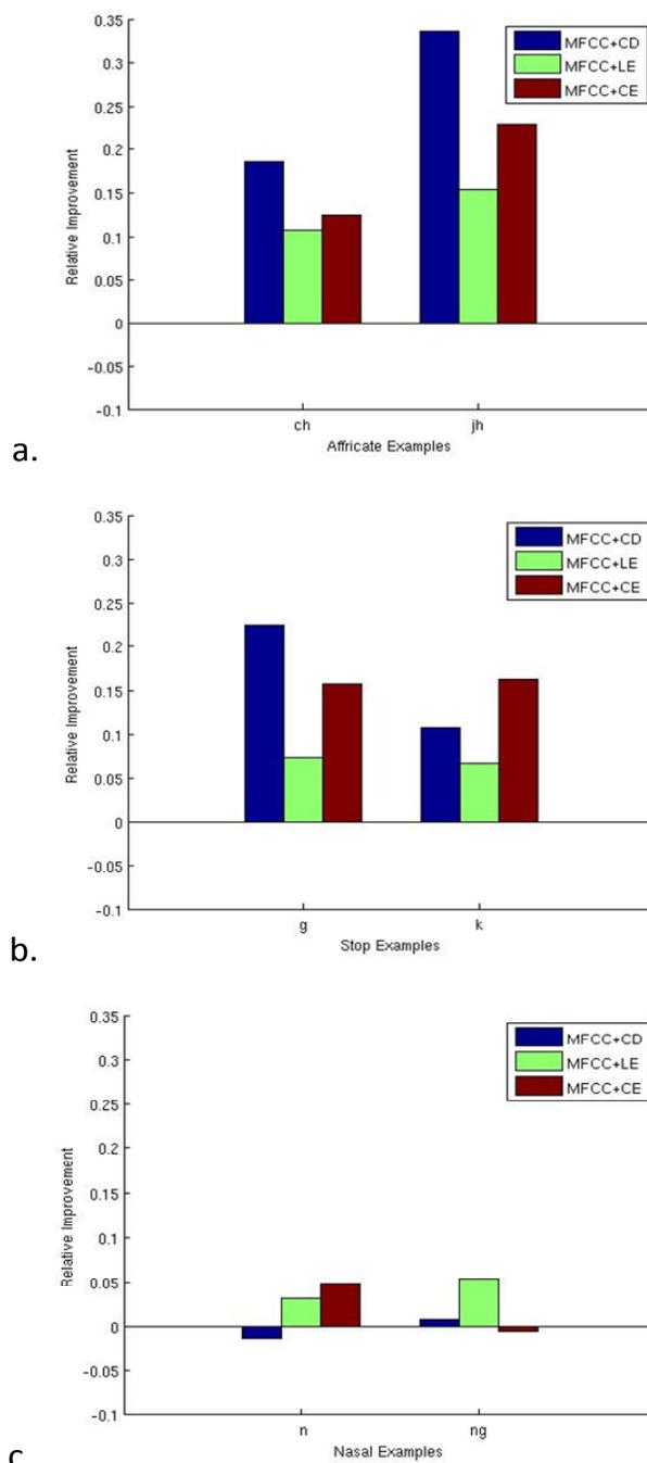
Figure 7. Relative improvements in recognition accuracy for several phonemes for an extended MFCC feature vector that includes nonlinear invariants (Affricates (a), Stops (b), Glides (c)).
