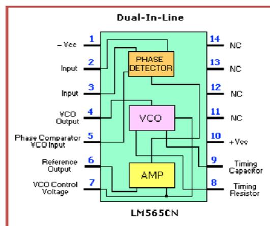
Figure 4. A phased-locked loop is a nonlinear device that is robust to unexplained variations in the input signal. Over time it synchronizes with the input signal without the need for extensive offline training [8].
