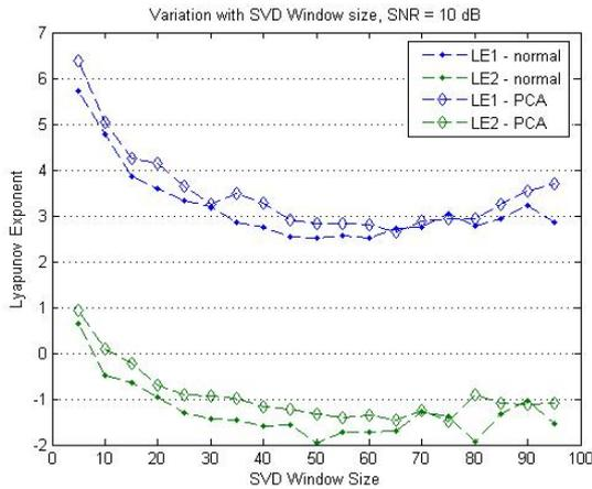
Figure 8 – Lyapunov Exponents from a scalar and a vector time series as a function of the SVD window size after PCA, SNR = 10 dB
