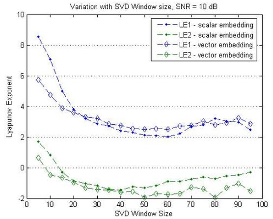
Figure 5 – Lyapunov Exponents from a scalar and a vector time series as a function of the SVD window size, SNR = 10 dB
