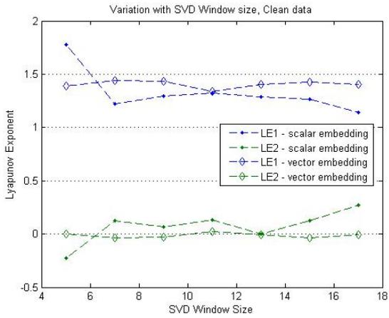
Figure 2 – Lyapunov Exponents from a scalar and a vector (clean) time series as a function of the SVD window length
